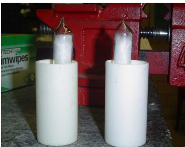
Fig. 6: Sealed growth ampoules in 50 ml \text{Al}_2\text{O}_3 crucibles for mechanical support. Note: in this image, the growth and catch crucibles are hidden by the 50 ml, support crucibles.
