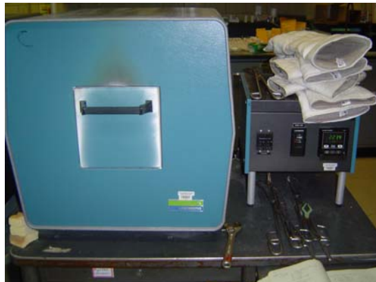
Fig. 8: 1500 °C, SiC heater element, box furnace used for solution growth. Power supply / temperature controller shown on right. High temperature gloves (on top of temperature controller) as well as tongs (on top and underneath of temperature controller) also shown.
