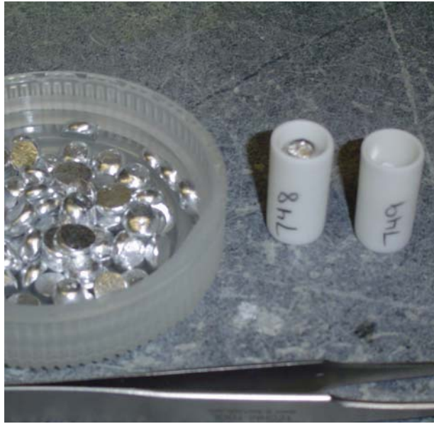
Fig. 3: \text{Al}_2\text{O}_3 crucibles being packed with elemental metals for growth of \text{RAl}_3 compound (elemental Al shown).
