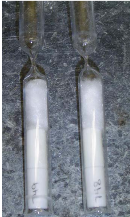
Fig. 5: Growth ampoules after necking, but before sealing. Note the silica wool above the catch crucibles
