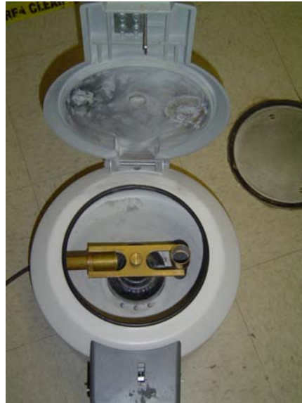
Fig. 9: Centrifuge with brass rotor and cups. Refractory fiber is used at the bottom of the sample cup to provide cushioning. Small coins of the world (as part of our international growth effort) are used as counter weights.
