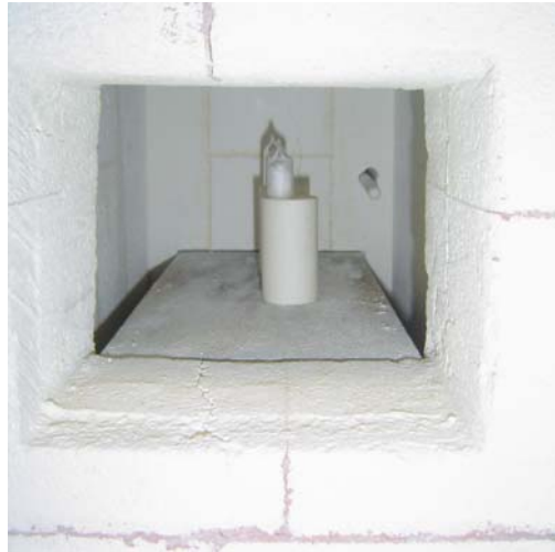
Fig. 7: Two growth ampoules in box furnace. Furnaces such as this can easily hold up to 10 growth ampoules and allow for rapid sampling of phase space
